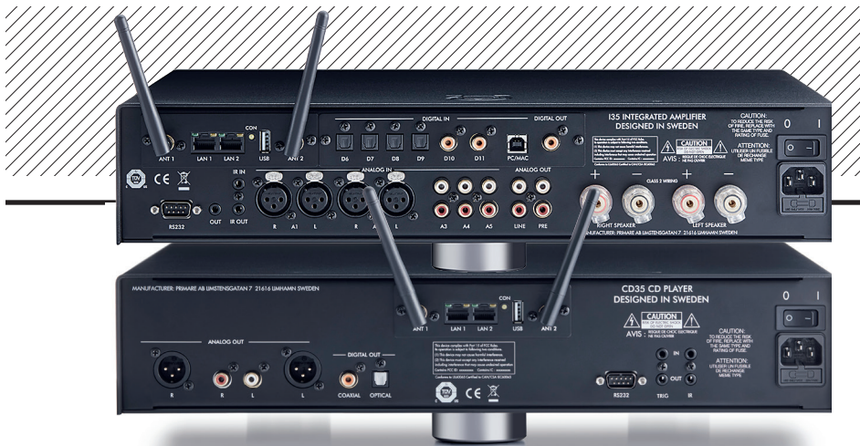
ABOVE: The amp [top] and CD player [bottom] include USB-A and Ethernet/Wi-Fi for Airplay, Bluetooth, Chromecast and Spotify. The I35 has four opt, two coax and USB-B digital ins alongside five line ins (two balanced on XLRs), pre out/line out and 4mm speaker terminals. CD35 includes balanced (XLR) line outs with coax/opt digital outs
